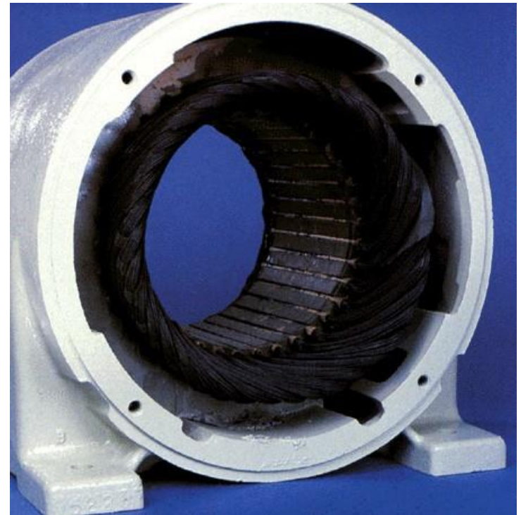
Motor Winding Damaged by Excessive Heat
